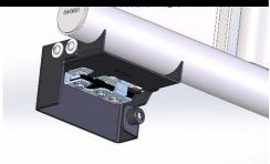
Mount the striker pin and mount as shown. Now you will need to adjust the latch and the pin so that the whole swing arm opens and closes nicely. You may also need to shim the rubber stopper closer to the bar for a proper latch.
